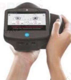
▲ **Spot vision screener finishes testing in less than 1 second.**
